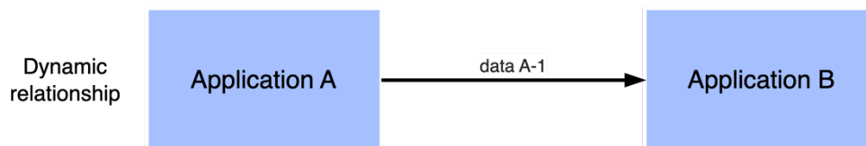
Figure 510: Dynamic relationship: application A transfers data (A-1) to application B.
